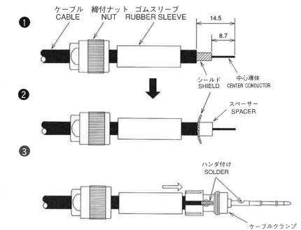
(3) Insert the cable into the cable clamp, leading the separated two shield conductors into both slits of the cable clamp. Butting the cable into the cable clamp softly, solder the center conductor. Trim the shield conductor to suitable length to be soldered shown, and solder them on the cable clamp as shown in figure (3). (Being soldered horizontally straight over the cable clamp as shown in this figure becomes stronger tensile strength.) Then, slide the rubber sleeve under the cable clamp.
